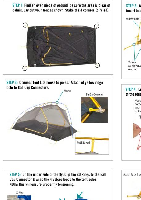
**STEP 2:** Assemble the "X" pole. Locate the YELLOW pole ends and insert into the corners with YELLOW SD Anchors/webbing.
