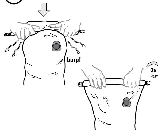
2. While holding the strips together, push down on sack to "burp" out trapped air. Tightly fold the top over a minimum of three times so that the gray sealing strip no longer shows.
